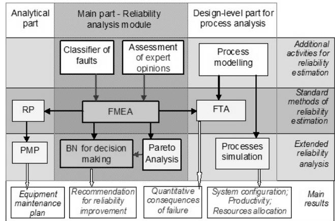
Fig. 1. Tool of a manufacturing process reliability assessment.
