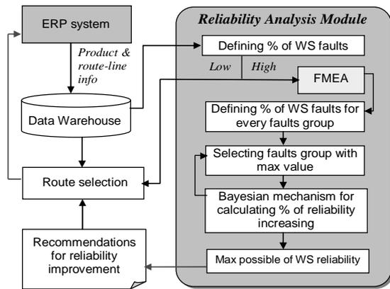
Fig. 3. Combination of a reliability analysis module and the ERP system for a production route selection.
