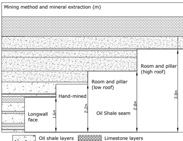
Using the results of the calculation method, it can be said that the undermined area in Kukruse-Tammiku secondary road region is mostly quasistable – it means the limestone layer and elements of the support were not broken during the extraction, but it may happen later [2].
