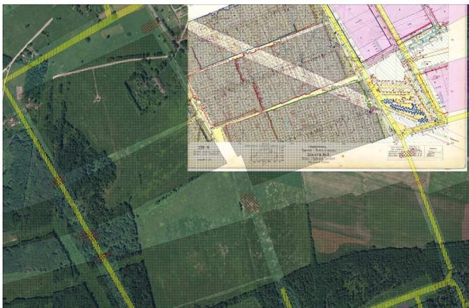
Fig. 1. Scanned mining plans, digitized mining plan and orthophoto.
