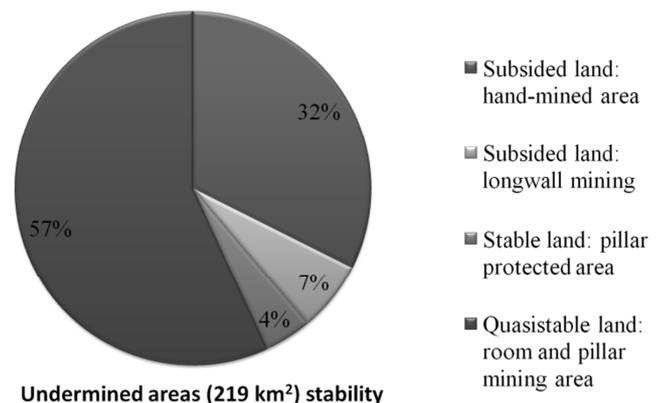
Fig. 2. Undermined areas stability in oil shale deposit.
