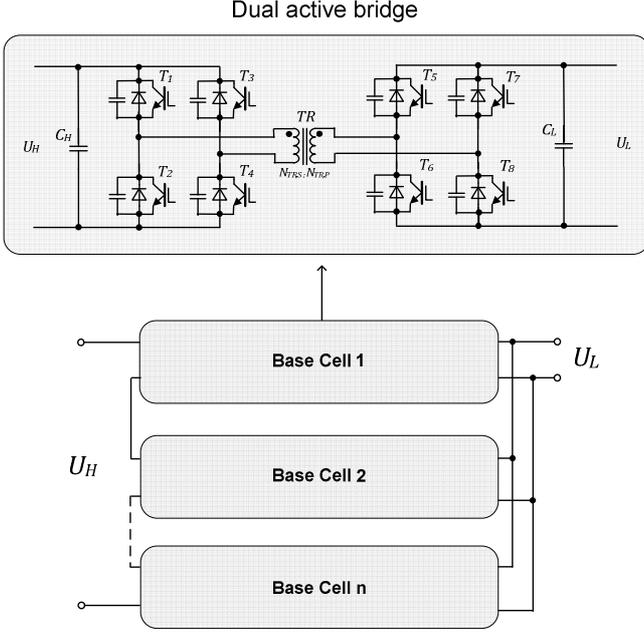
Fig. 1. Modular structure of power electronic transformer with DAB based isolation stage.
