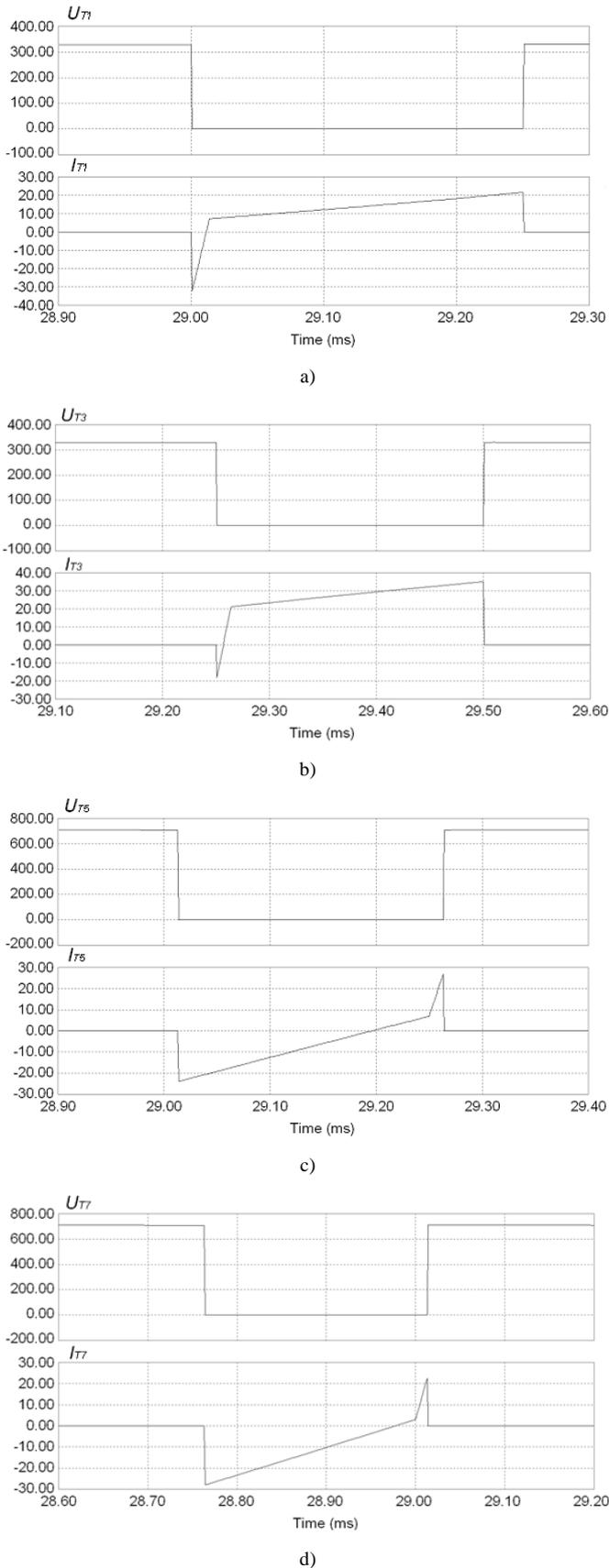
Fig. 3. ZVS sequence of the DAB all four legs: a – primary leading leg; b – primary lagging leg; c – secondary leading leg, d – secondary lagging leg.
