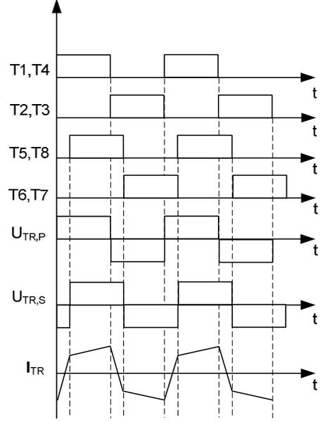
Fig. 2. Gate signals, transformer primary and secondary voltages, as well as transformer current waveforms.
