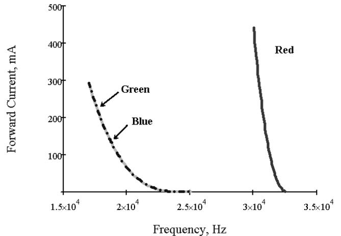
Fig. 6. Different color LED forward current dependence from frequency for CZFM control method at 5V input voltage and constant zero state time  $t_{off}=20\mu s$ .
