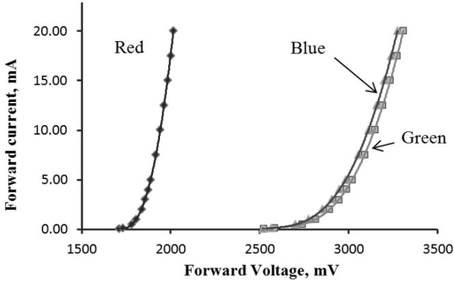
Fig. 2. Current-voltage curves of RGB LED for separate color chips (utilized in experiments LED).
