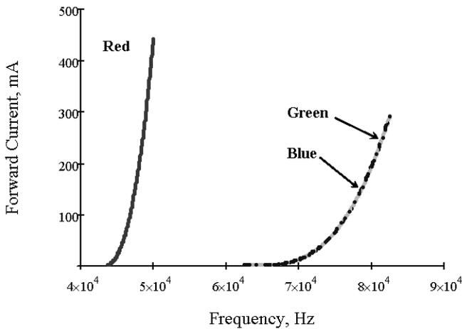
Fig. 5. Different color LED forward current dependence from frequency for CPFM control method at 5V input voltage and constant positive pulse time  $t_{on}=8\mu s$ .
