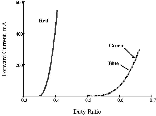
Fig. 4. Different color LED forward current dependence from duty ratio for PWM control method at 5V input voltage and constant frequency.
