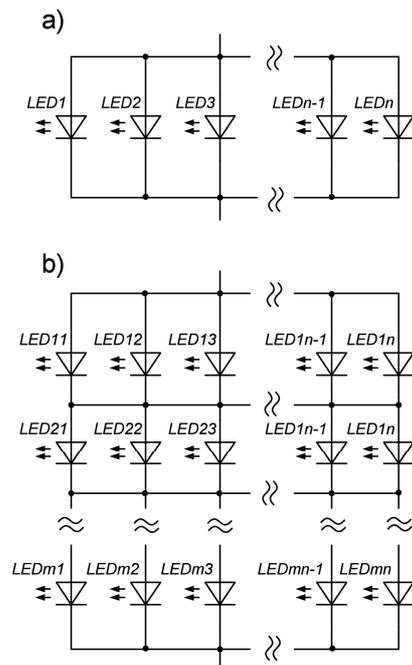
Fig. 3. Principal schematics of chip connections in high power LED: a) parallel connection; b) matrix connection.
