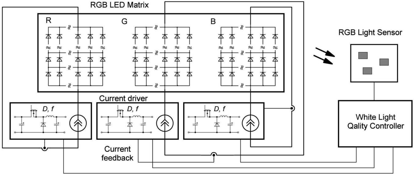
Fig. 7. Block schematics for control system of RGB high power LED.
