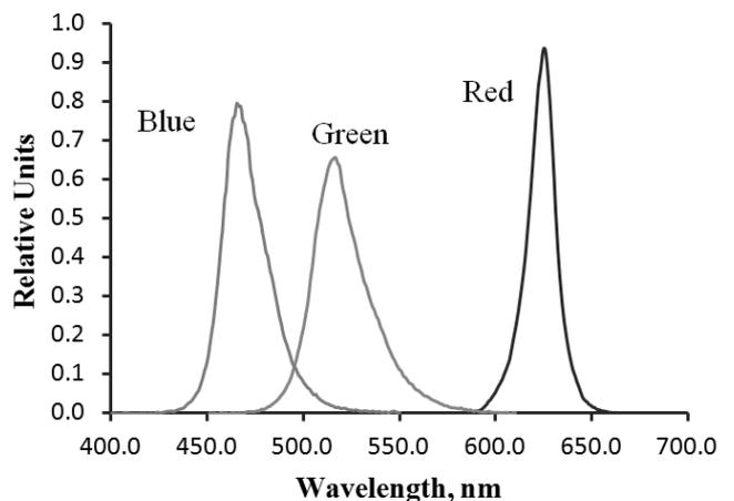
Fig. 1. Spectral distribution of RGB LED used in experiments.
