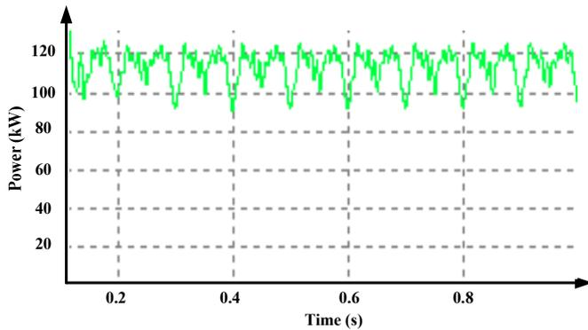
Fig. 15. Line power waveform with PCS compensation.
