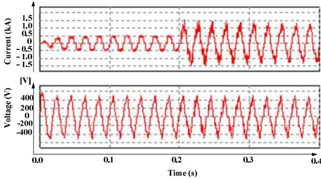
Fig. 2. Load current and inter-phase voltage measured in typical grid.
