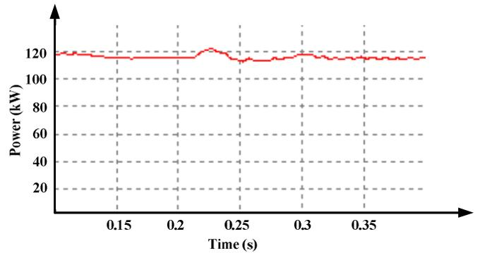
Fig. 12. Power of the line after compensation by PCS.
