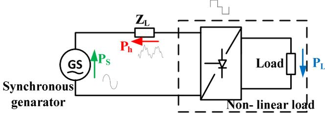
Fig. 1. Power flow in system with non-linear load.
