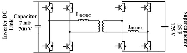
Fig. 6. DC/DC converter
