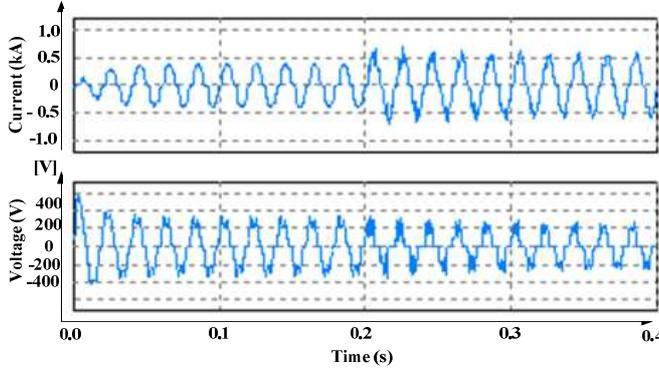
Fig. 3. Load current and inter-phase voltage measured in “soft” grid.
