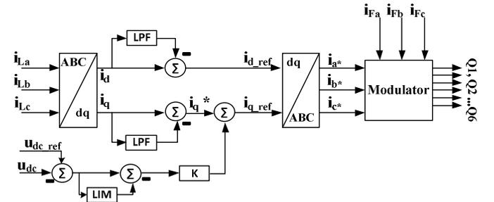
Fig. 5. Control structure of the proposed PCS.
