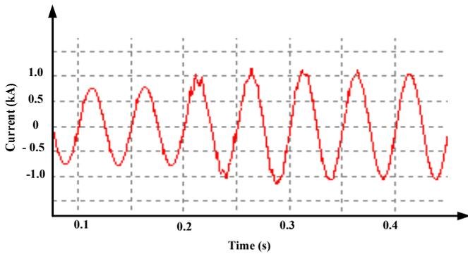
Fig. 9. Line current after compensation by PCS.
