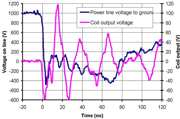
Fig. 7. Testing results with non-loaded coil.
