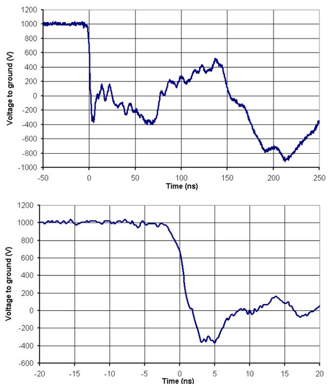
Fig. 1. Voltage variation on high voltage line upon ground fault. Upper – overview; lower – close-up view of transient.
