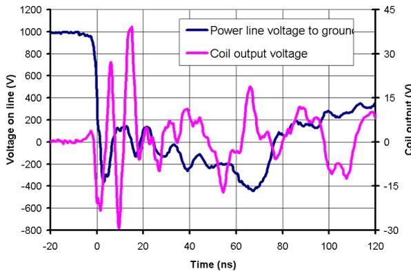
Fig. 8. Testing results with coil loaded with 330 ohm resistor.
