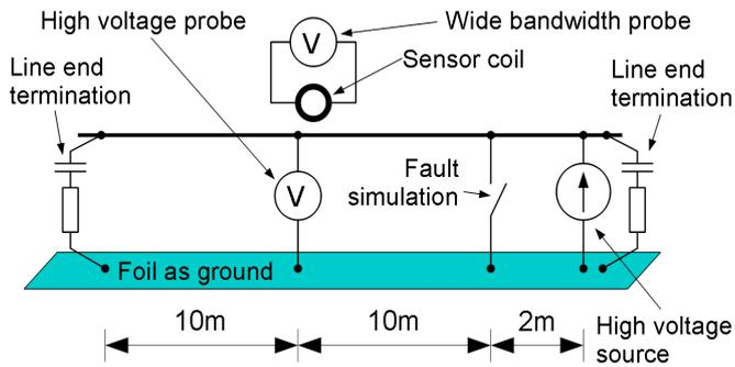
Fig. 2. Testing set-up of traveling wave measurements.
