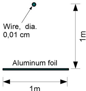
Fig. 4. Testing power line set-up.
