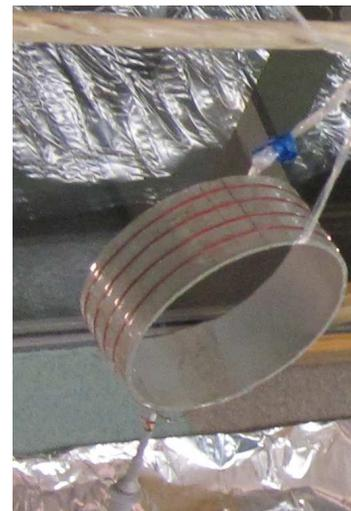
Fig. 6. Coil used for testing assembled to the line. In the bottom oscilloscope probe is visible.
