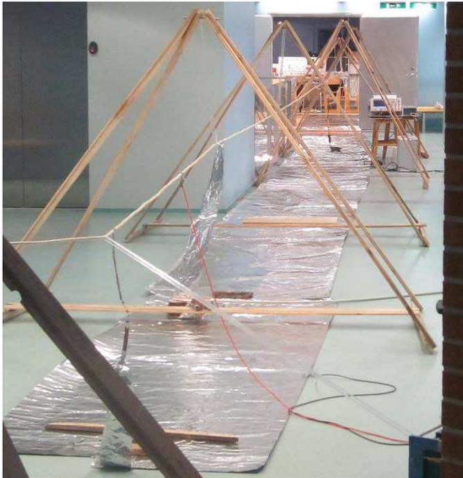
Fig. 3. Testing set-up of traveling wave measurements.
