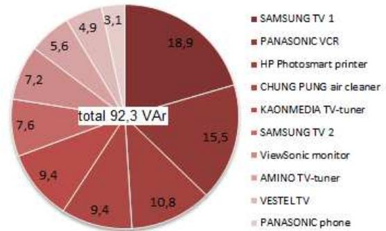
Fig. 2. Reactive power of devices at standby mode in vars.
