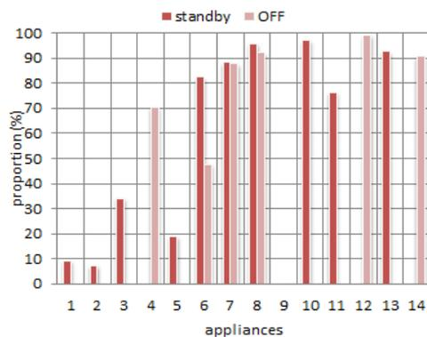
Fig. 6. Standby/ OFF mode reactive power proportions to ON mode value.
