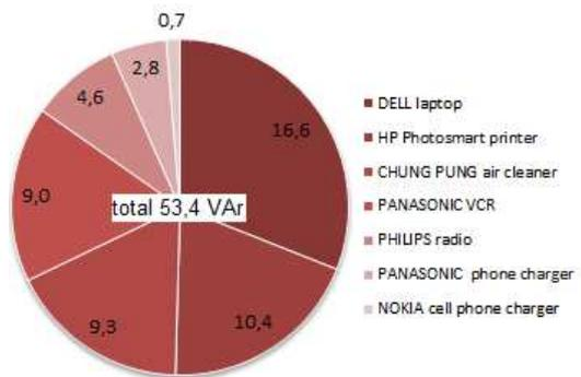
Fig. 4. Reactive power of devices at OFF mode in vars.
