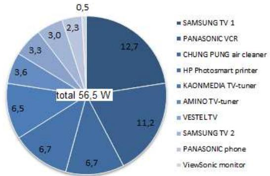
Fig. 1. Active power of devices at standby mode in watts.
