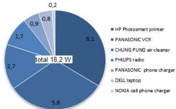
Fig. 3. Active power of devices at OFF mode in watts.
