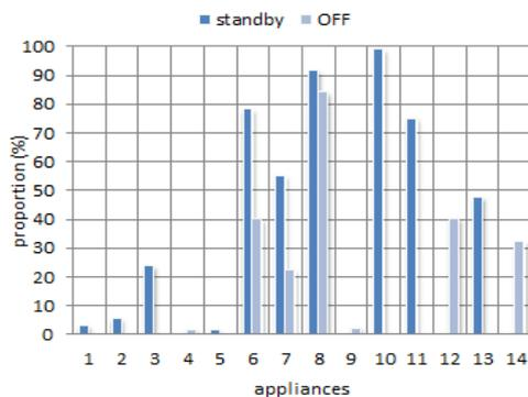
Fig. 5. Standby and OFF mode active power proportions to ON mode value.
