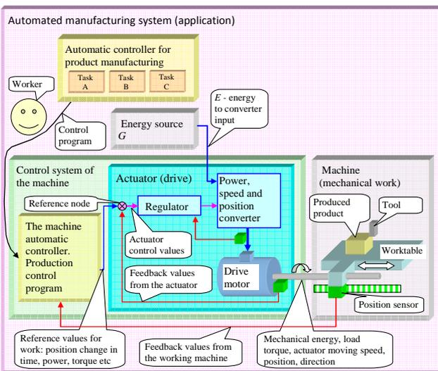
Fig. 1. Structure of an automated manufacturing system [8].
