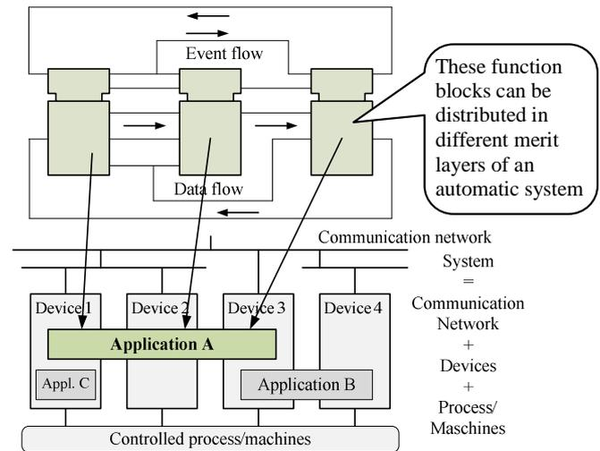
Fig. 11. Overview of the standard 61499 function block model and architecture.
