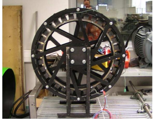
Fig. 11. Prototype machine with ferrite magnets.
