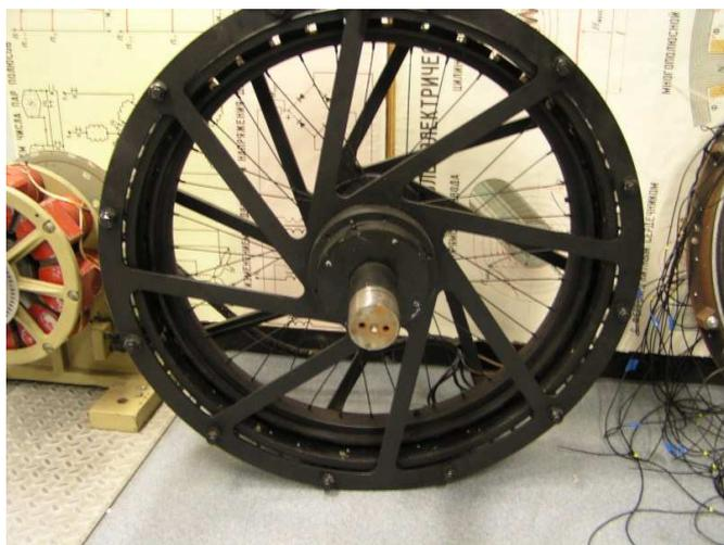
Fig. 6. Prototype machine with NdFeB magnets.
