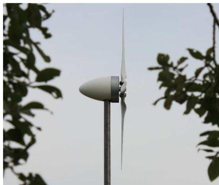
Fig. 8. Prototype downwind windmill.
