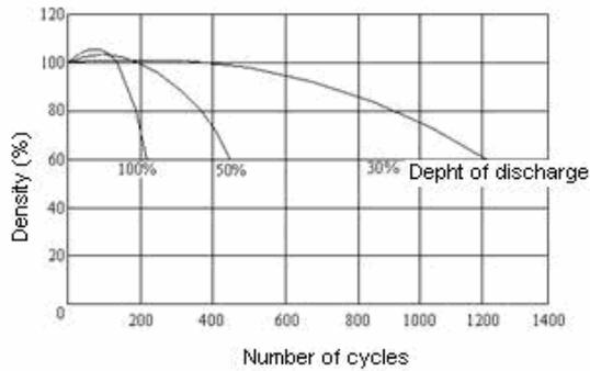
Fig.2. LAB Lifetime versus depth of discharge
