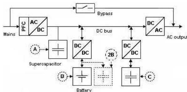
Fig. 6. Topology of on-line UPS
