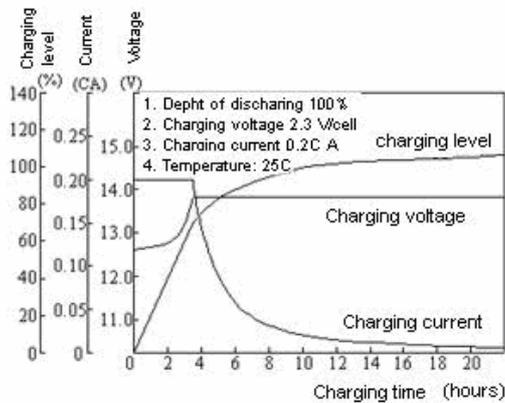
Fig.3. Charging current of a LAB
