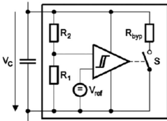
Fig. 5. Topology for active voltage balancing
