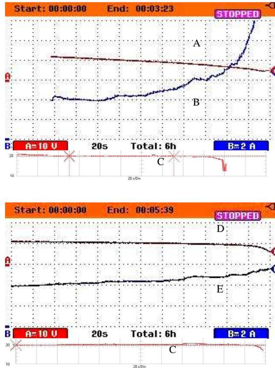
Fig. 7. Discharging characteristic of battery and supercapacitor (A – supercapacitor voltage, B – supercapacitor current, C – DC-bus voltage, D – battery voltage, E – battery current).
