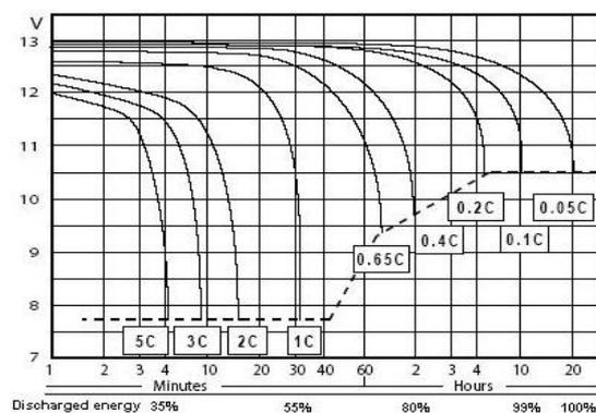
Fig.1. Discharge characteristics of a LAB
