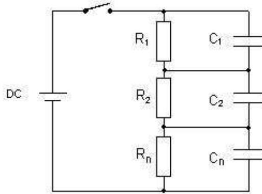
Fig. 4. Topology for passive voltage balancing
