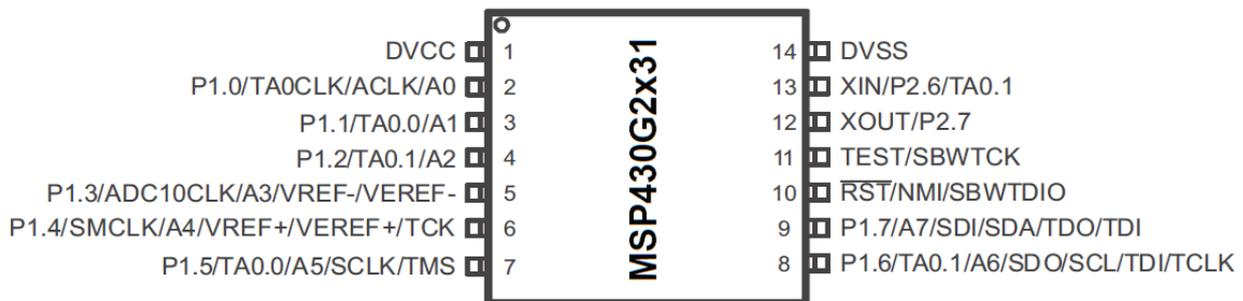
Figure 7. Pinout of MSP430G2231
